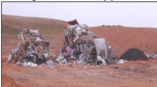
Figure 9 : Classic image from Lancaster County Solid Waste District in PA Comparing the Disposal of MSW at landfill and the 90% reduction of Ash from the processing of MSW at WTE [7]
